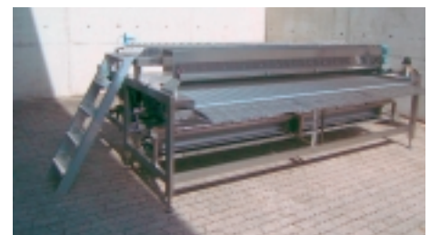
igubal® flange bearings as drive bearings in a conveyor system for bakery products
