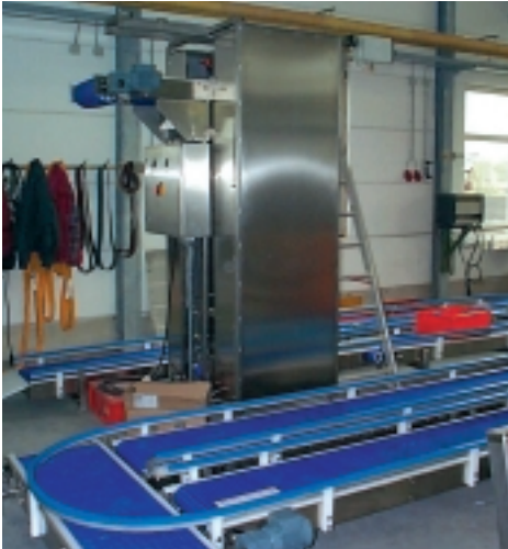
Igubal® pillow block bearings in conveyor systems for the food industry (see pictures at the right for details)
