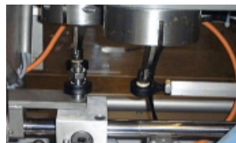
igubal® rod end bearings in a candy decorating machine
