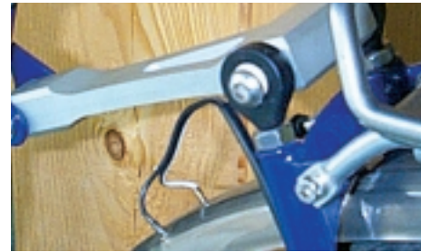
igubal® rod end bearings in the spring loaded rear axle rocker of a bicycle
